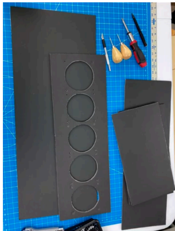
From Left to Right: excess foam core, Fan Panel, Top and Bottom Panels, Back Panel.
